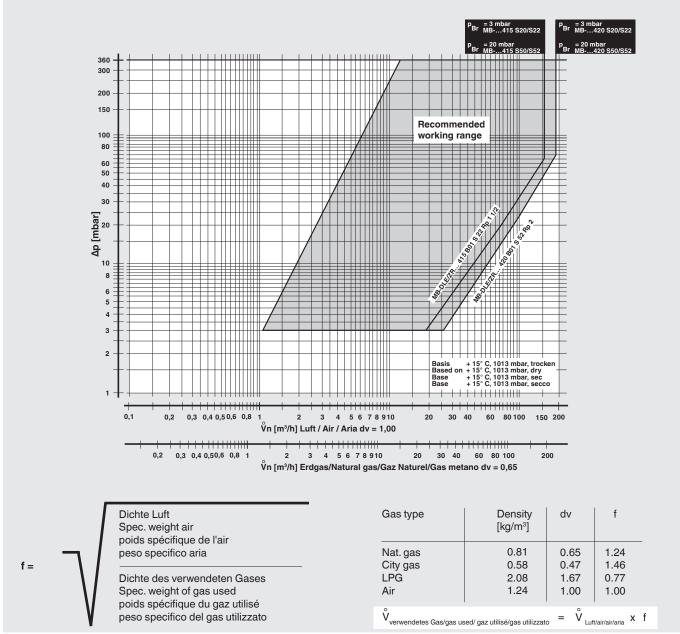
Volumetric flow pressure loss characteristics in regulated state with microfilter
